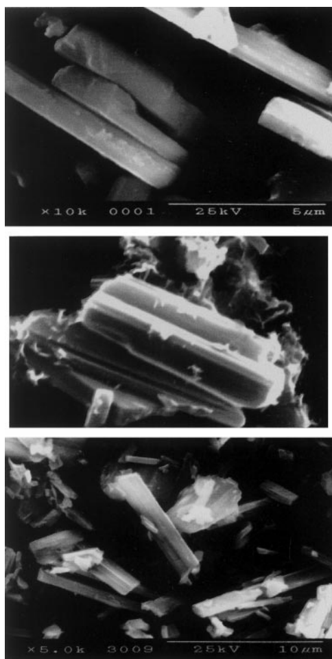
FIG. 3. SEM images of \text{LiMnO}_2 (top), \text{MnO}_2 \cdot 0.70\text{H}_2\text{O} (middle), and \text{MnO}_2 \cdot 0.22\text{H}_2\text{O} (bottom).
